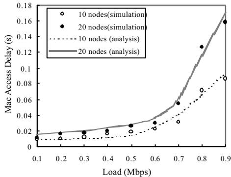
Fig. 3 Access Delay in Single-Hop Scenario
